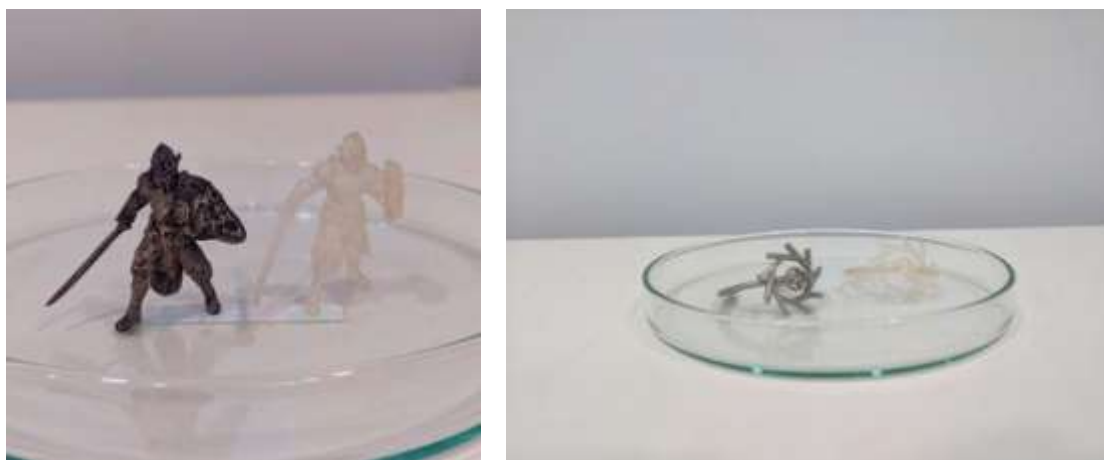
Figure 2. 3D printed artifacts of complex geometry before and after their metallization.
