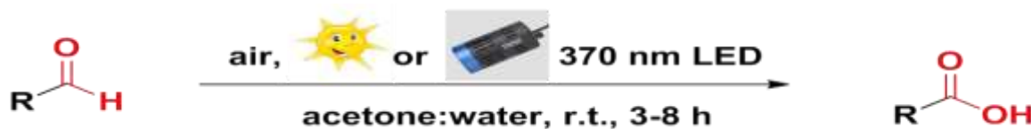
Figure 1. Light-mediated aerobic oxidation of aldehydes to carboxylic acids.
