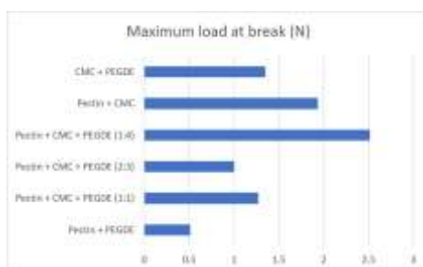
Image 2: Tensile strength of different pectin films tested.
