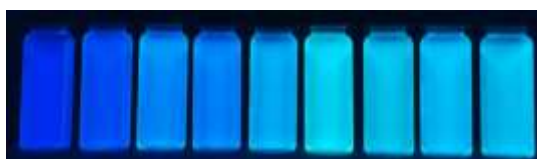
Figure 3: Fluorescence of pyrrole in different solvents (from left to right: CH, Toluol, THF, EA, \text{CH}_2\text{Cl}_2 , DMSO, ACN, iPro, EtOH under UV-lamp, c = 10^{-5} mol/L, \lambda_{\text{exc}} = 365 nm).
