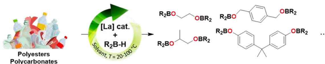
Figure 26. Our catalytic system for the reductive depolymerization of polyesters and polycarbonates
