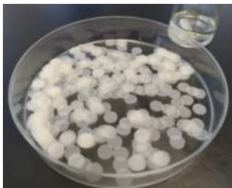
Figure 1. PVDF membranes impregnated with NADE.
