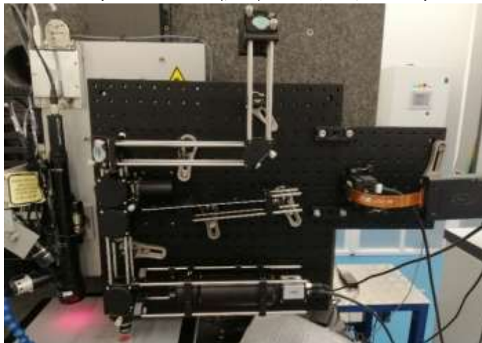
Figure 21 Optical setup for TPP available at AIMEN facilities
