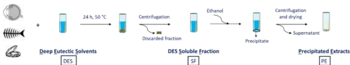
Figure 1. Bioactive extraction process.
