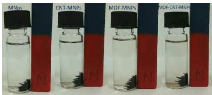
Figure 2. The magnetic behavior of the synthesized materials.
