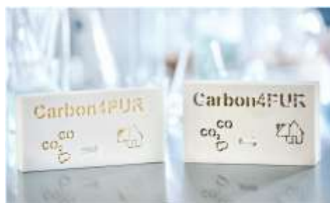
Figure 1. Rigid PIR-foams on lab-scale utilizing Carbon4PUR polyol made from CO-derived SA produced by carbonylation and commercially obtained SA.
