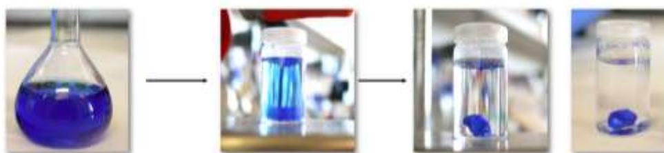
Figure 1 –Schematics of the adsorption experiments, where the initial and final aspect of the PIL and the aqueous dye solution can be observed.
