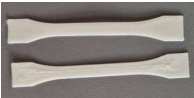
Figure 1. FFF 3D printed samples used in seawater durability tests.
